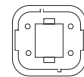
G24Q 4-PIN BASE (NOT INTENDED TO REPLACE 2-PIN G23 OR GX23 2-PIN LAMPS)
